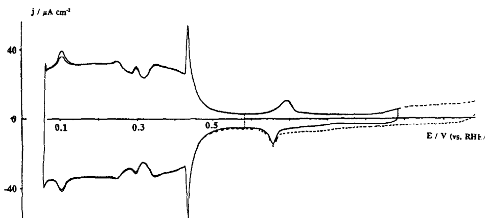
Fig. 6. Highly reversible surface process of electrochemical H adsorption and desorption at a Pt (111) surface in aqueous 0.1 M \text{H}_2\text{SO}_4 (298 K), illustrated by the 'mirror-image' cyclic voltammogram. (The anodic and cathodic currents correspond to the H adsorption pseudocapacitance, C_\phi = i/s .) Pt (111) flame-treated electrode after cooling in air, and sweep rate = 50 \text{ mV s}^{-1} .
